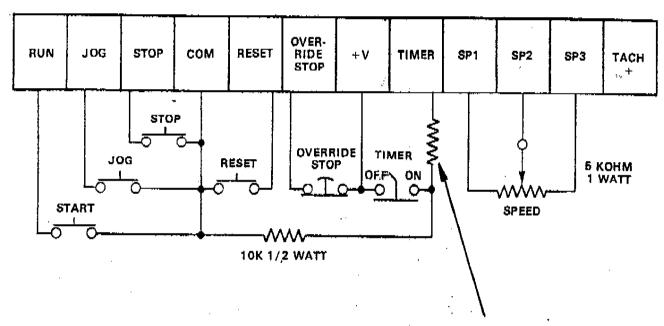
The external timing resistor can be a fixed resistor, or a potentiameter, or a combination of both. The resistance required can be approximated from the formula  $R = \frac{T}{0.015}$
